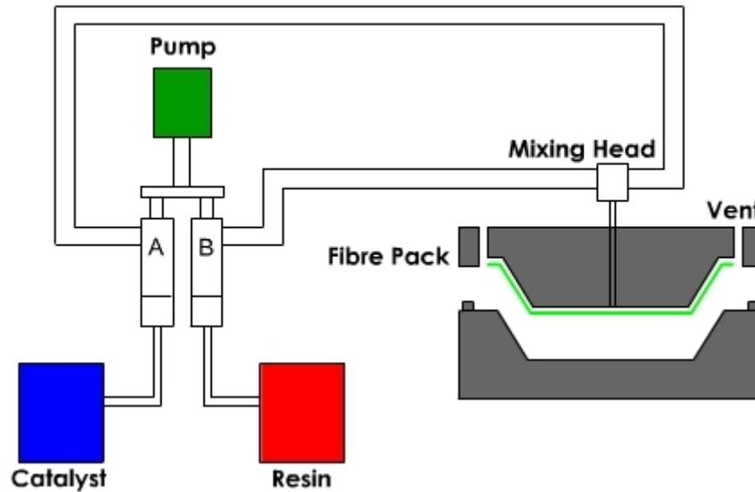
A. FIBRE LOADING AND MOULD SETUP
