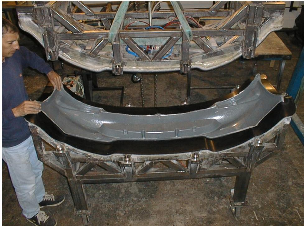
MOULD OPENED AFTER RESIN INJECTION
