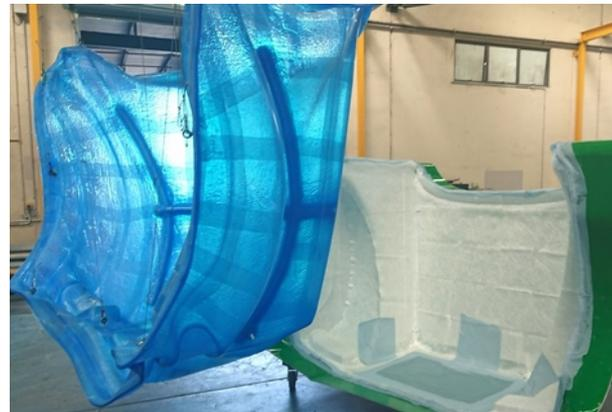
Flex RTM – Male Mould is made of Silicon
